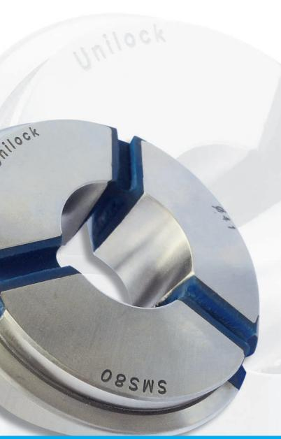
**SMS clamping collets** are made up from metal inserts, units of vulcanised rubber. This allows the collet to close radially in a perfect manner, blocking the piece along the entire length of the hole and eliminates the intrusion of shavings to pass inside the spindle.
